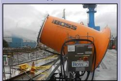
Dust Suppression Units are used to mitigate the escape of dust from sandblasting operations in the drydock.
