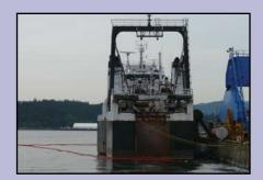
An orange inshore containment boom fully surrounds the vessel while being fuelled.
