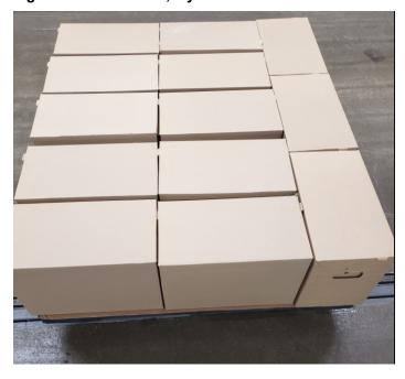
Figure 2 Skid of B20's Layout for rows 1 & 3
