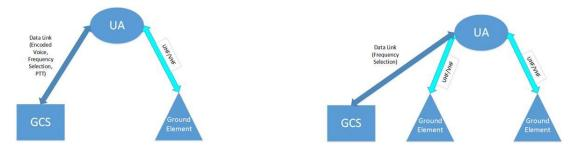
A33. The requirement is to relay VHF and UHF radio broadcasts to ground elements within range. This means that VHF and UHF broadcasts can be passed to other elements within range of the UA. It is not intended to be VHF and UHF broadcasts from the GCS to the ground element.
