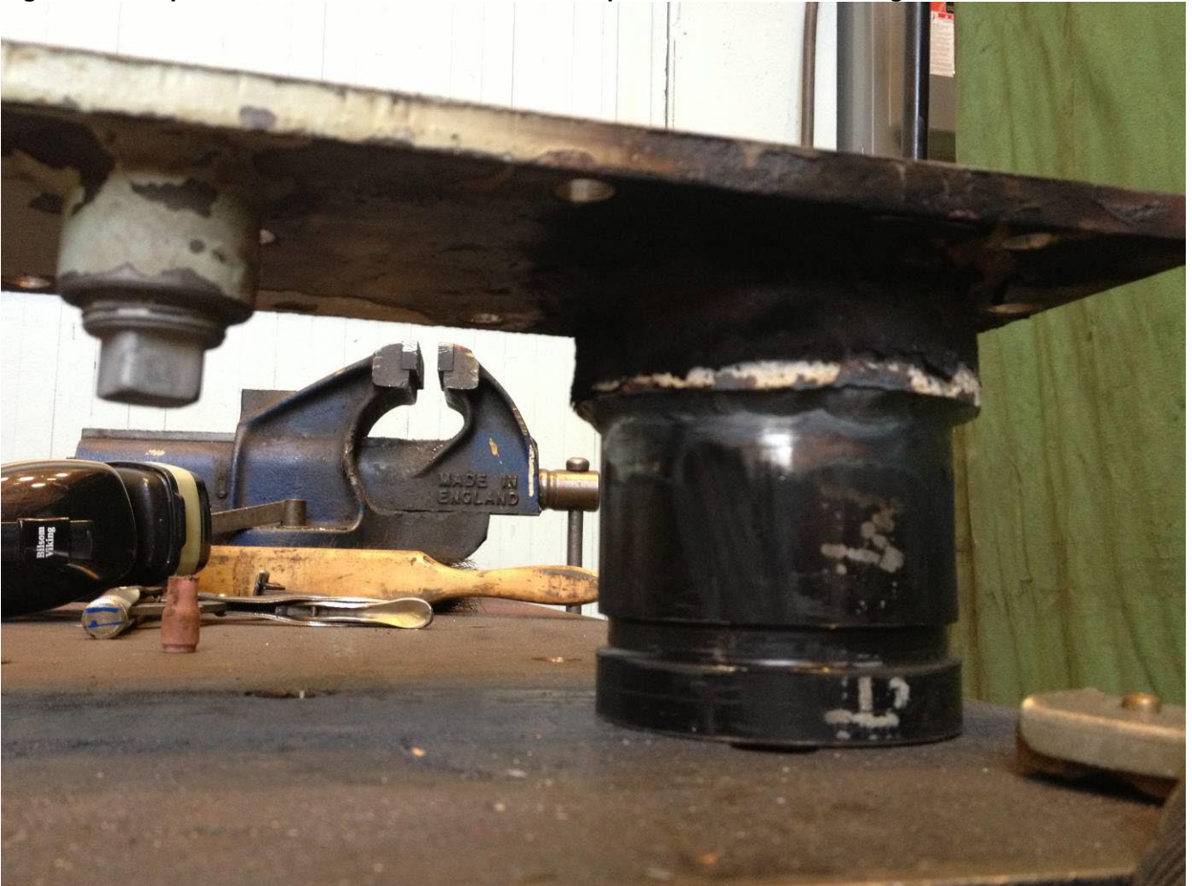
Figure 7: Example of a Manifold Fitted with a New Adapter for 3" Grooved Fittings
