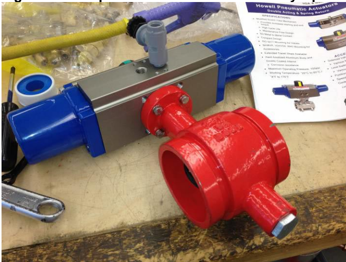
Figure 9: Example of a 3" Grooved Pipe Adapter Ready for Welding to a 3.5" Branch of the 8" Drain Line.
